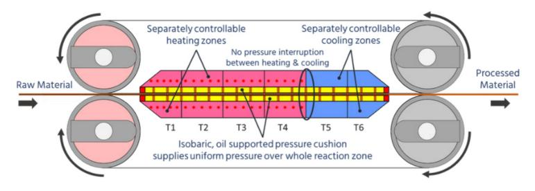
At the intake and the outlet, the steel belts are looped around heated steel drums.
